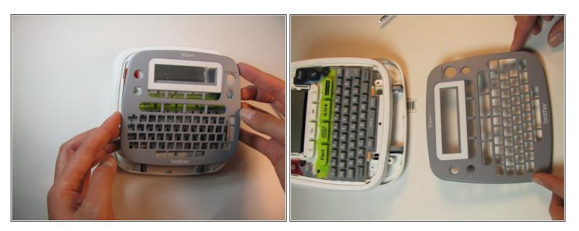
• Pull the clips inward two at a time, first the top then the bottom, to snap the face plate off.
