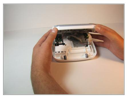
• Close the back cover and then flip the device over and separate the top half from the bottom half as shown.
