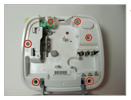
Use the Helping Hand 1/4" screwdriver to unscrew the six 3/16" corner screws.
