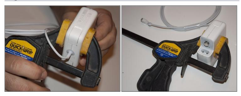
• Clamp the casing together and give it a few hours for the glue to set.
