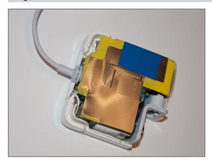
Put the cord winding flappers back in position.
