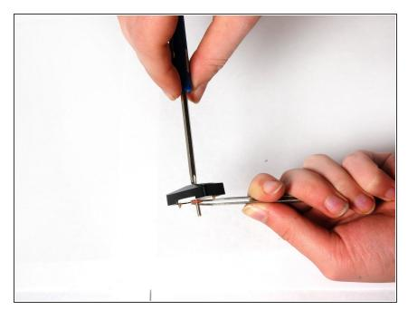
Hold on to the red disc with needle nosed pliers, and use the Phillips head screwdriver to remove the disc by pushing down.
