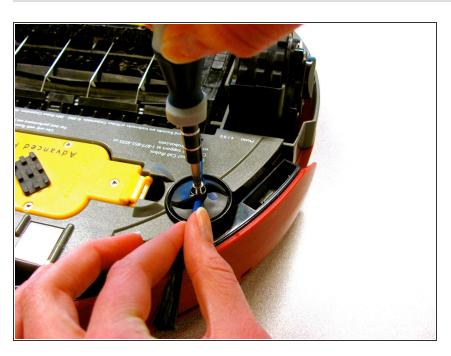
Using the Phillips #1 Screwdriver, unscrew the 7.2 mm Phillips #1 screw while holding the edge brush in place.
