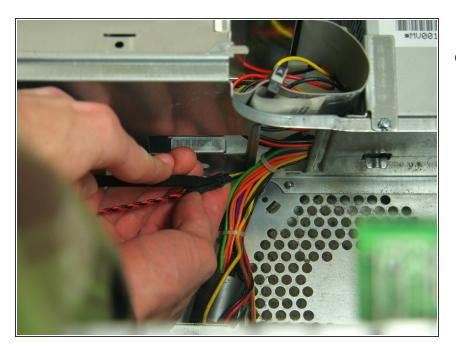
Remove the power cable from the fan and detach bracing.
