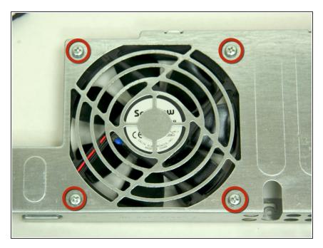
To fully remove the fan, unfasten the 4 screws on the front of the bracing using the Phillips #2 screwdriver.
