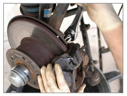
Then tighten the bolts down until they seat against the caliper. Do not tighten them all the way down with the normal ratchet wrench.
