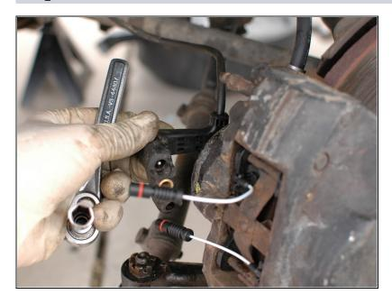
Re-attach the sensor harness and insert the sensors back in to the connectors on the harness.
