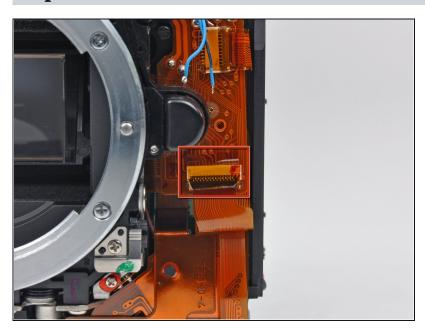
i If present, remove the piece of tape covering the ribbon cable socket (boxed in red).
