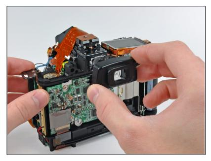
• Carefully remove the eyepiece from the D70.
