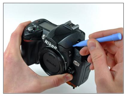
Use a plastic opening tool to carefully pry up the flash unit at the point shown in the picture.
