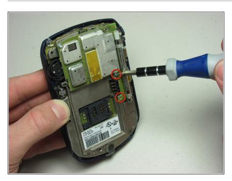
Remove the two T6 screws.
