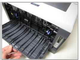
Located on the back of the printer, open up the cover by grabbing onto the tab and pulling down.
