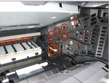
⚠ DO NOT TOUCH the electrodes on the right inner wall of the printer. Touching these electrodes can cause electrical damage to the printer.
