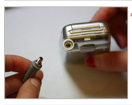
Make sure that the threads line up when screwing the new antenna back on, otherwise a strong connection won't be made.
