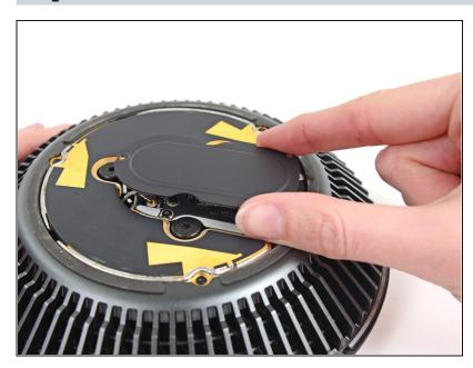
• Lift and remove the metal cover from the AirPort board bay.
