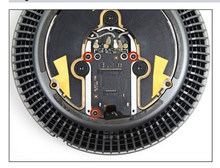
Remove three 3.7 mm T4 screws securing the AirPort board to the fan assembly.
