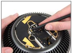
• Use the tip of a spudger to disconnect the four AirPort antenna cables from the AirPort card.
