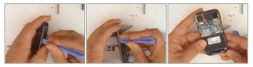
After removing the back housing you must disconnect the antenna cable, the LCD connector and unstuck Vol(+,-) keys. There is another one screw. Now you can remove the main-board.
