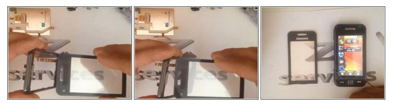
• Install new touch screen and assembly the phone.
