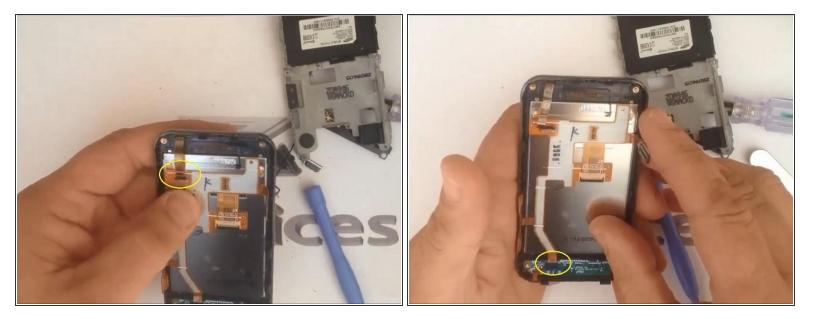
Disconnect the flex-cable from touch screen and the flex-cable from the small keyboard down.
