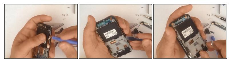
Unstuck camera keys and remove the middle bezel.
