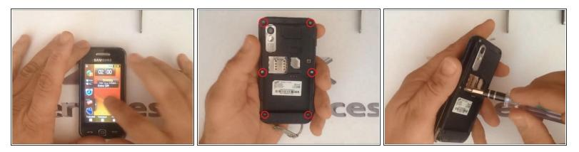
Remove the battery, the SIM card and the memory card. Then you must unscrew 6 phillips screws.
