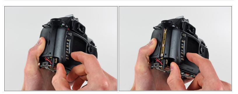
• Carefully pull the sides of the rear cover away from the body of the D70.
