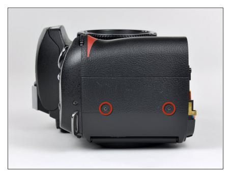
Remove the two 4.8 mm Phillips screws securing the battery side of the rear cover to the D70.
