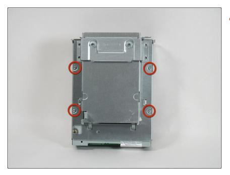
• Remove the four screws holding the enclosure to the drive.
