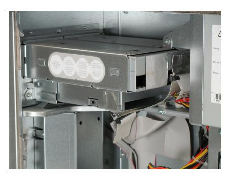
• The optical drive is in the top left corner of the case.
