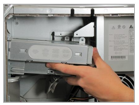
Remove the optical drive by pulling the drive away from the front of the computer and out.
