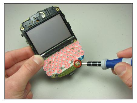
• Remove one T6 Torx screw in the front bottom right of the board.
