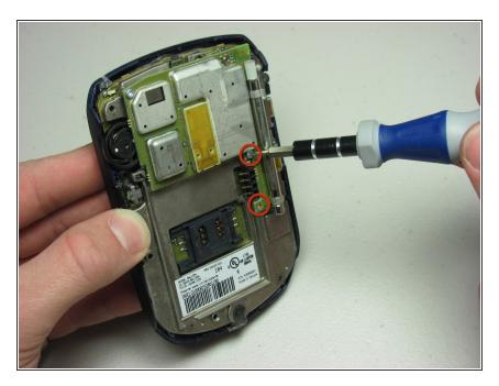
• Remove the two T6 screws.
