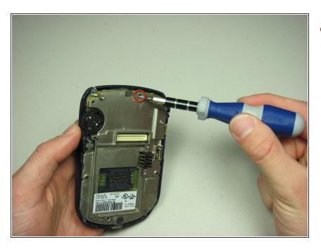
• Using the T6 Torx screwdriver, remove the top screw.
