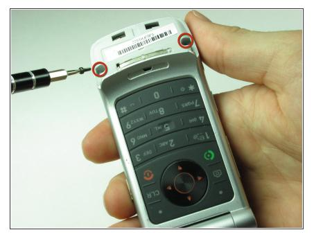
• Remove the two Torx-6 screws under the removed plastic.
