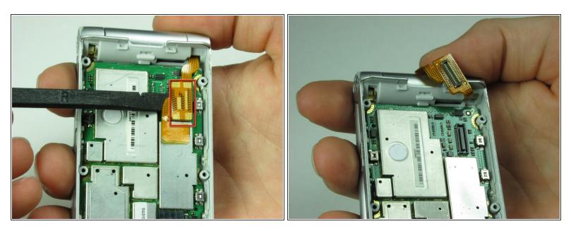
Use spudger to gently separate the ribbon cable from the logic board.
