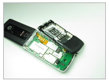
• The casing can be easily removed exposing the bottom logic board.
