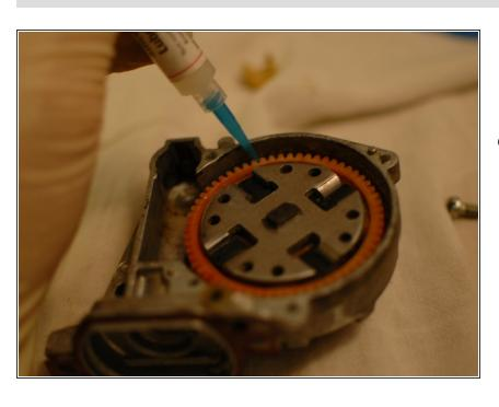
Once dry, grease the large plastic gear and the worm gear on the motor with a synthetic grease such as silicone based SuperLube. Avoid petroleum greases such as vaseline or moly grease as they can damage plastic and rubber parts.
