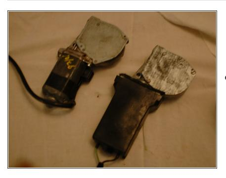
Before starting this guide, confirm that you are reviewing the guide for the correct motor type for your situation. This guide covers the "Drill Open" style of motor, as seen on the left. If you have a "Screw Open" style of motor as seen on the right click here to review this guide instead.
