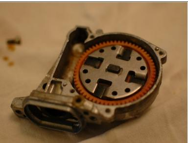
Use a de-greaser to carefully clean the entire gear housing to remove any metal shavings and old grease. Rinse thoroughly and then air dry.
