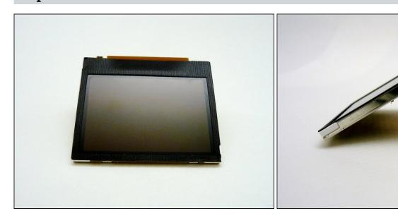
• The LCD can now be cleaned or replaced.
