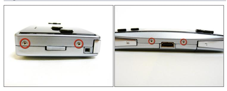
• Remove the two tri-wing screws on the top of the Game Boy and the two screws next to the volume/contrast switch.
