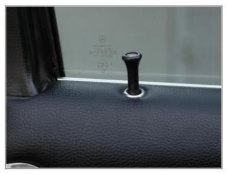
• Begin by removing the door lock knob. It unscrews counter-clockwise.
