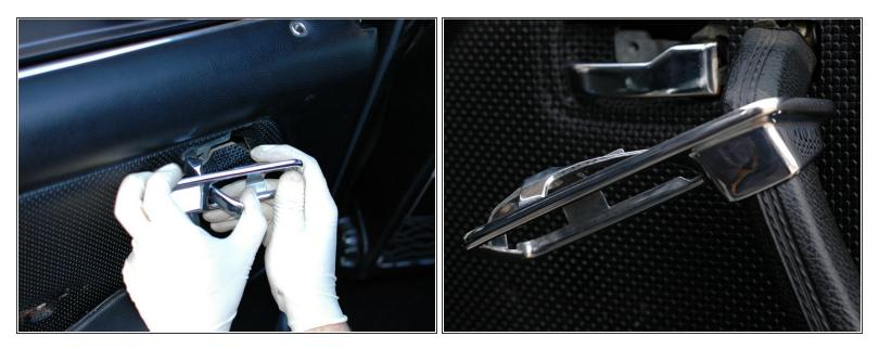
• On the other three doors, the chrome panel is a part of the upper arm on the door panel. Pull the chrome panel out from behind the door pull. You will need to pull the door pull away from the door to get the chrome panel around it. It will move down the arm on the door panel.
