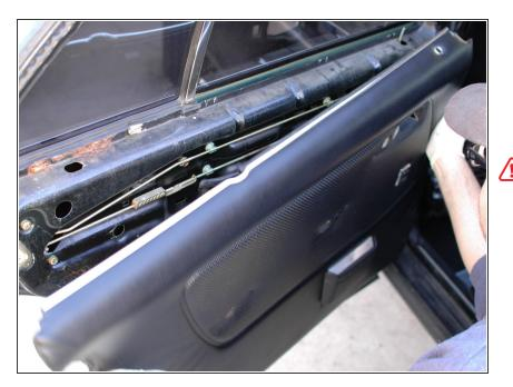
Remove the panel by pulling up on it. Do not pull straight out on the panel, or it may bend. This cannot be repaired. Pulling up on the panel before pulling out on it will also help ensure that you do not damage the plastic clips on the back of the map pocket on the door panel (only applies to front panels; rear panel shown in this picture).
