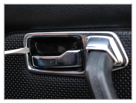
Use a flat blade screwdriver to gently pry out the black plastic cover behind the door pull.
