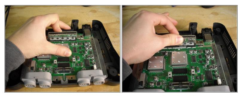
Detach the current slot from the motherboard. To do this, simply pull at the cartridge slot located in the center at the rear of the console. Rock it back and forth and pull upwards until it detaches. Be careful of the pins connected at the bottom. These will need to be wired to the motherboard, so do not damage them.
