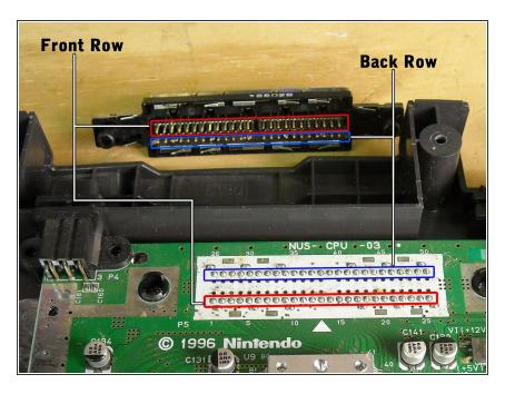
Start by soldering one end of the 2inch wire to the left-most pin on the disconnected cartridge slot, and the other end of the wire to the left most contact point on the motherboard.
