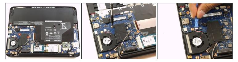
• Remove the two Phillips screws on the fan.
