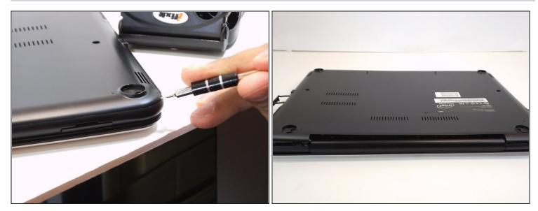
• Loosen the back cover panel using a spudger.
