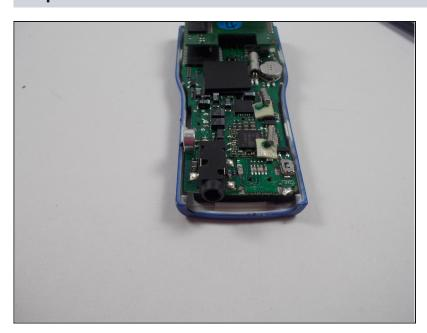
Align the new headphone jack appropriately on the motherboard for soldering.
