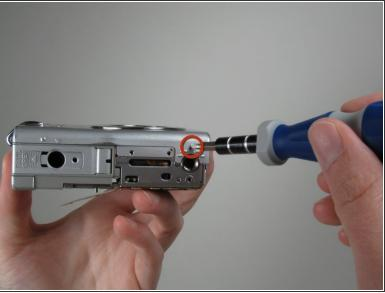
Unscrew the four Phillips screws from the side of the casing and one screw from the bottom using a #0 Phillips screwdriver.
