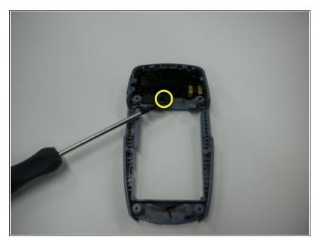
On the bottom casing, there should be a single metal screw holding the antennae in. Remove this screw.
