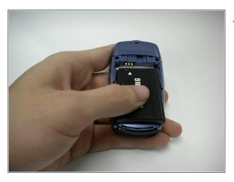
Pull the battery up from indent at the bottom and slide it out.
