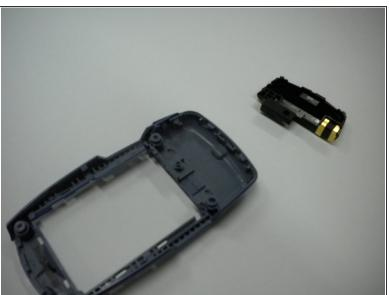
Pry the antennae off by inserting a flat object such as a spudgel into the slot marked in yellow and pushing upwards.
