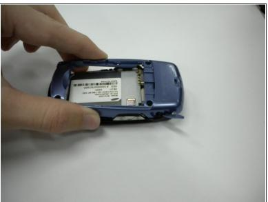
Use a spudger to pry the back assembly off of the device.
