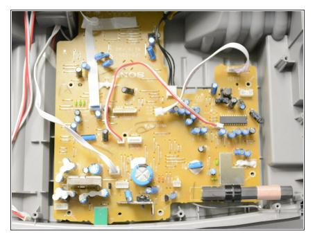
Insert and align the new circuit board and screw it down.
