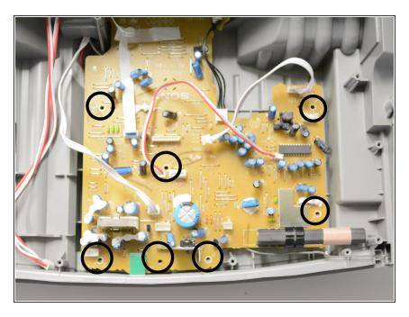
Unscrew the screws in the circuit board.
