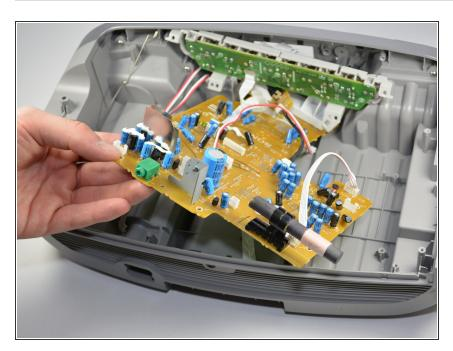
Lift the circuit board out of the radio.
