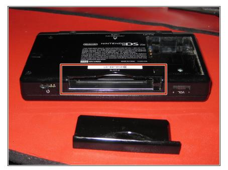
On the front edge of the Nintendo DS between the headphone jack plug and volume controls remove the plastic insert (or cartridge) from the lower slot (Slot 2).
