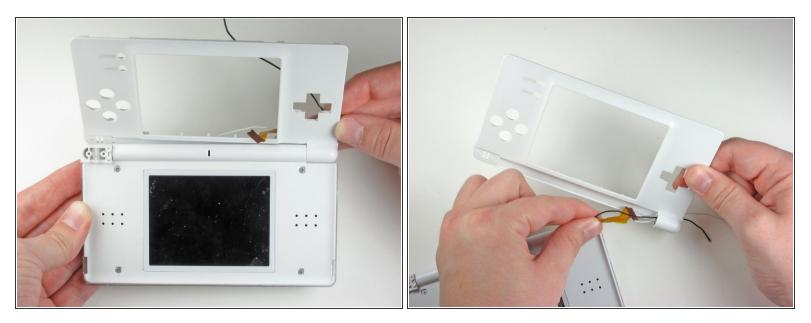
After opening it, carefully unhinge them from each other by sliding the bottom piece to the left and the top piece to the right.
