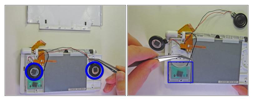
• Carefully remove the two speakers and the green wireless card from the top panel.
