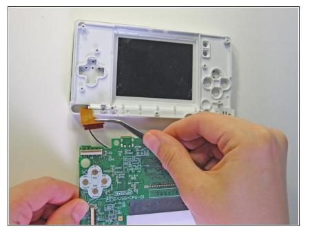
Using one finger nail or the plastic opening tool, carefully lift the brown securing flap of the connector. Then disconnect the ribbon cable that connects the logic board to the upper screen.
