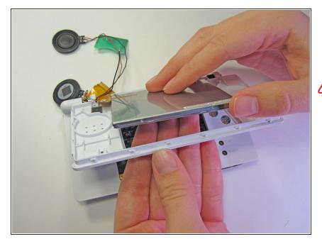
Remove the screen by orienting it face down and pushing up on the screen from underneath.
