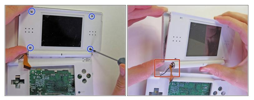
Unscrew the four Phillips-head screws and remove the top panel.
