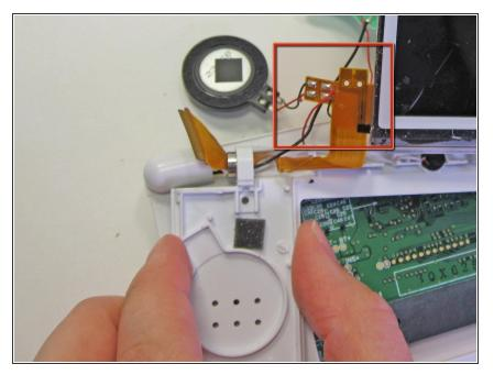
• The speakers are soldered to the top screen flex assembly. You may desolder a broken speaker and solder a working speaker on, or you may replace the speakers together with the display assembly.
