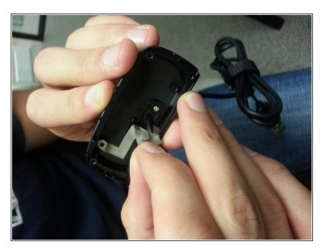
Remove PCB from the base plastic piece.
