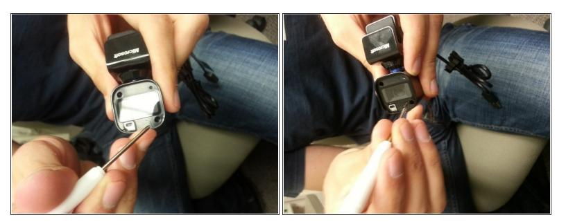
Once frame is taken off the front, two screws need to be removed.
