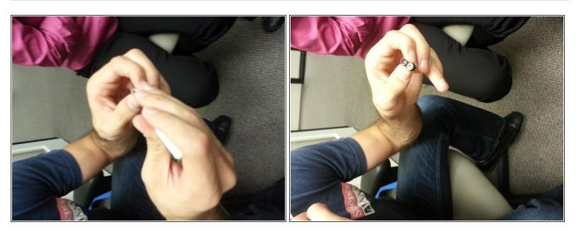
Take out the IR filter by using a scalpel for pulling out the lens tape.
