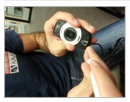
Remove cover to get to the PCB underneath
