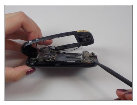
Using the spudger, remove the inner case from the phone.
