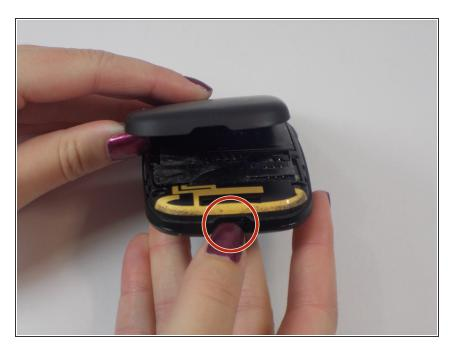
Push in the button at the bottom of the phone, and lift the back cap off.
