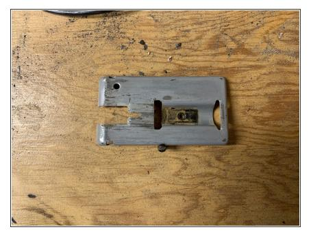
After removing M4 screw, remove the base plate and place to the side. Don't forget to replace the M4 screw near the base plate during reinstallation.
