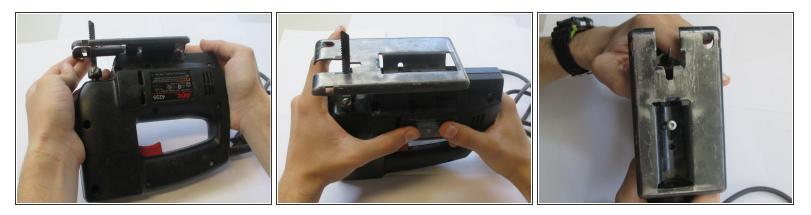
Orient your saw so that the blade is pointing in the opposite direction of your body. Ensure that the screws circled are visible and pointing skyward. This will be the standard position of the Jigsaw for the duration of this guide.
