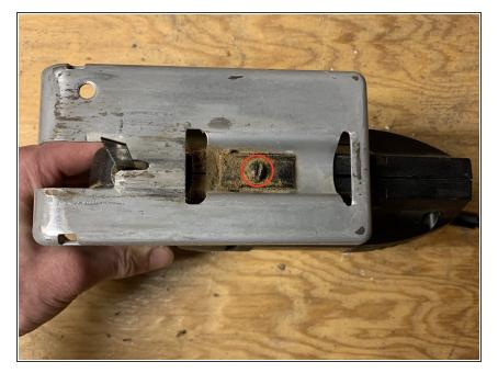
• With bottom of the base plate visible, identify one M4 screw circled in red and remove with Phillips screwdriver (some models have flathead screw, as pictured, and require flathead screwdriver).
