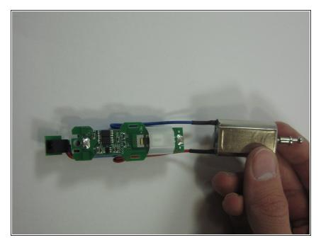
Remove the motor, battery, and motherboard from the plastic casing.
