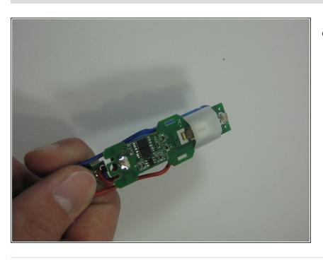
Remove the old motherboard and install the new one. Then, connect the wires and white piece to the new motherboard.
