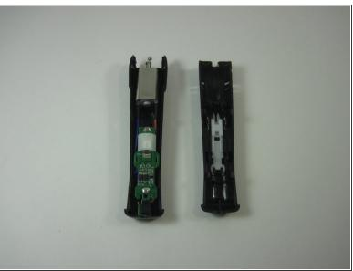
Pry open the plastic cover into two separate pieces. The plastic is very durable so don't worry about breaking it upon prying it open.
