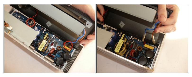
Caution: The circuit board contains many capacitors that could cause serious injury if touched. If possible, use a <u>capacitor discharge probe</u> to safely rid the capacitors of dangerous charges.
