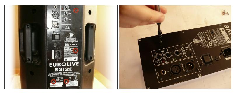
• Remove the 4, 7/32" long machine screws with a #2 phillips head screwdriver.
