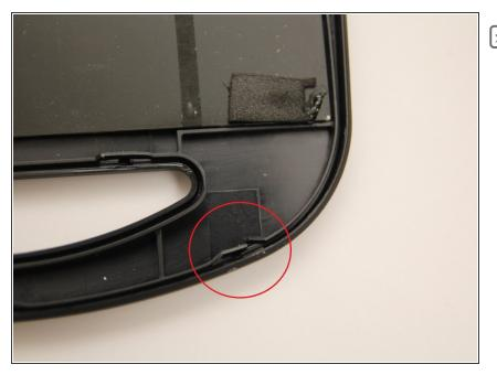
Here is an example of a broken clip to remove the panel.
