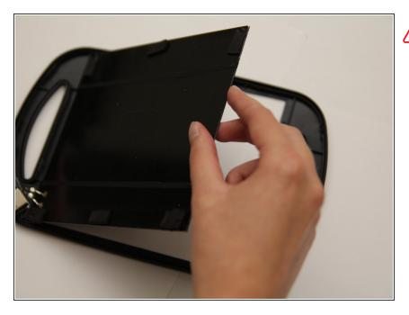
The only thing holding the solar panel in place now is gravity, so make sure not to flip the device over! This may damage the connections.
