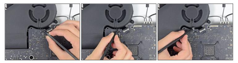
• Use the tip of a spudger to disconnect the fan cable's connector from its socket on the logic board.
