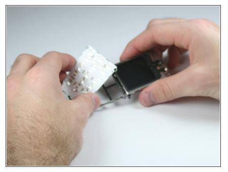
• Lift the keyboard out of the plastic frame.
