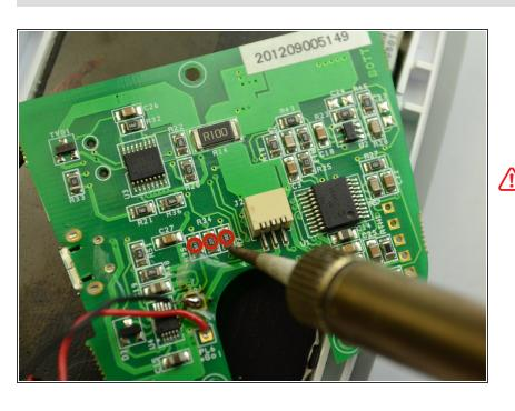
↑ Soldering can melt key components and cause harm to both the user and the device. Read soldering
