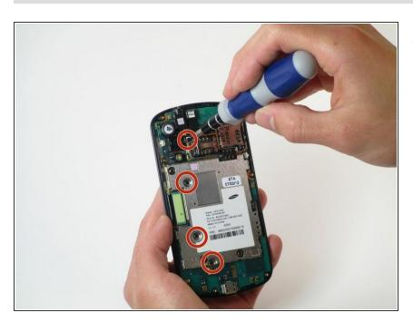
Remove the four black 3mm screws securing the motherboard with the Phillips #000 screwdriver.
