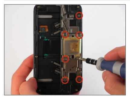
Remove the 7 silver 2mm screws attaching the silver metal plate to the rear panel with the Phillips #000 Screwdriver.
