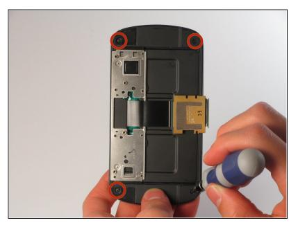
Unscrew the 4 black 3mm screws from the rear panel with the Phillips #000 Screwdriver.
