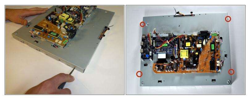
• Unscrew the 4 5mm Phillips PH2 screws on the sides of the monitor.
