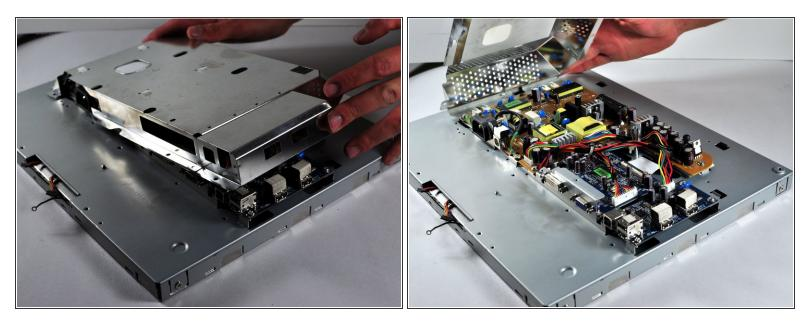
• Pull the the metal casing off of the monitor to reveal the motherboards.
