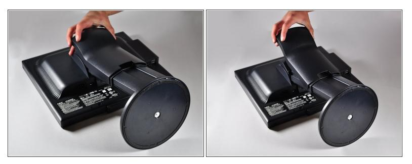
• Firmly remove the back panel of the stand by pulling it up and away from the monitor.
