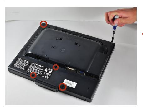
With the monitor face-down, unscrew the 5 7mm Phillips PH2 screws around the outside of the enclosure.
