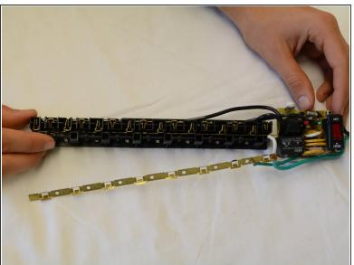
Lift power plugs out of bottom of case along with circuit assembly
