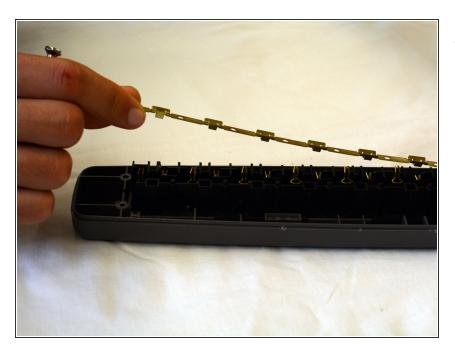
Lift Ground Copper Strip upward off of power plugs by hand
