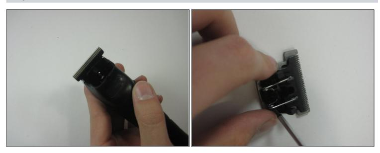
• Apply pressure to the back side of the blades while pushing outward to remove the blade head completely from the Wahl Lithium Ion Trimmer.
