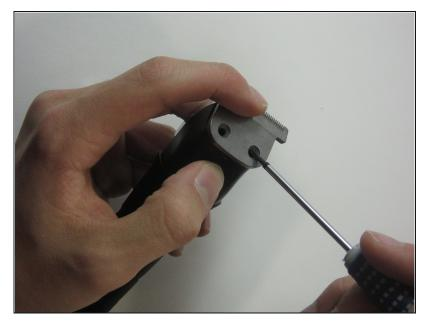
• Unscrew the two Phillips screws that hold the blades in place with a Phillips #0 screwdriver.
