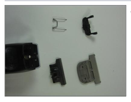
Separate the Wahl Lithium Ion Trimmer head into its four components. Remove the damaged blade and replace it with a new one.
