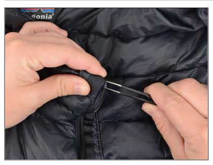
Carefully remove any remaining pieces of the stop using <u>tweezers</u>.
