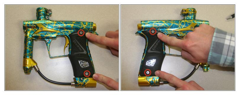
• Remove the four screws from the grip with the 5/64" allen wrench. There are two on each side.
