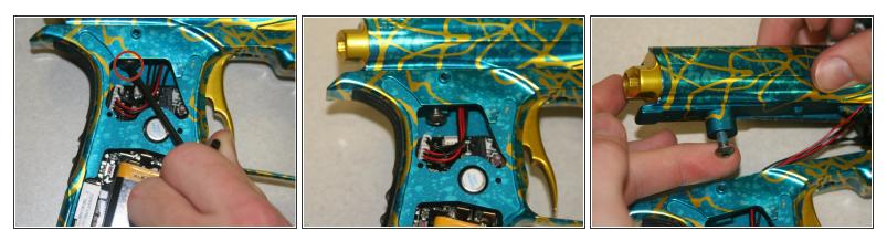
Use 1/8" allen wrench to loosen the screw inside the grip on the right side. *(i)* The screw only needs to be turned a couple of times.
