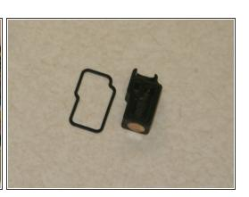
Remove the solenoid gasket manifold by applying pressure with one finger to the part closest to the end of the barrel.
