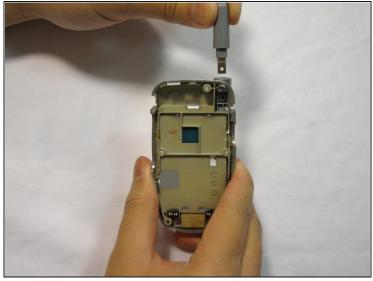
• Remove the copper fixture after it has been unscrewed.
