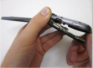
• Lift the back cover starting at the bottom of the phone.
