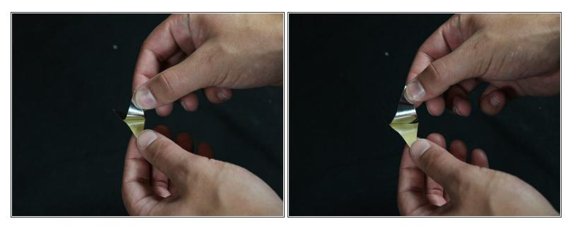
• Peel the reflective foil off of the cut piece.
