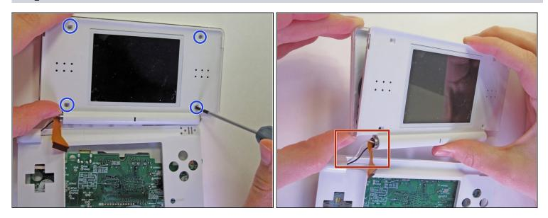
Unscrew the four Phillips-head screws and remove the top panel.
