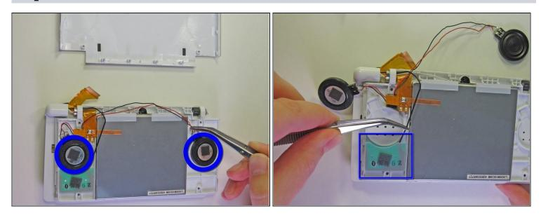
• Carefully remove the two speakers and the green wireless card from the top panel.
