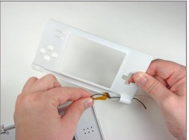
• After opening it, carefully unhinge them from each other by sliding the bottom piece to the left and the top piece to the right.
