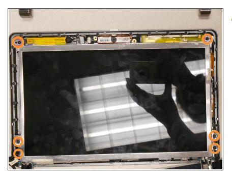
Remove the six (6) 5mm screws shown here using the Phillips #0 screwdriver.
