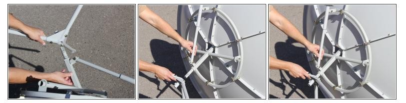
• Attach the top of the center plate of the tripod base stand to the cross bearer bar making sure the flat side of the tripod legs points away from the solar panel dish.
