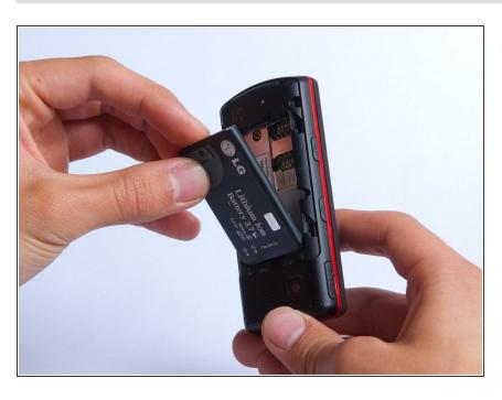
Lift and remove the battery.
